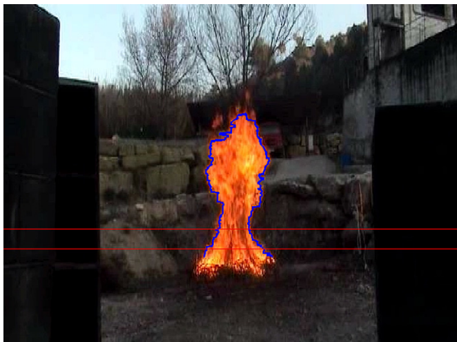
Fig. 4. VHS image of an arbitrary time instant of the QI field test that shows the flame contour extracted to compute flame thickness. The red lines indicate the part of the flame vertically covered by the radiating panels. (For interpretation of the references to colour in this figure legend, the reader is referred to the web version of this article.)
